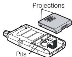
1. Align the projections on the battery pack with the pits on the transceiver.
