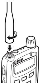
1. Connect the helical antenna to the antenna connector at the upper left corner.
